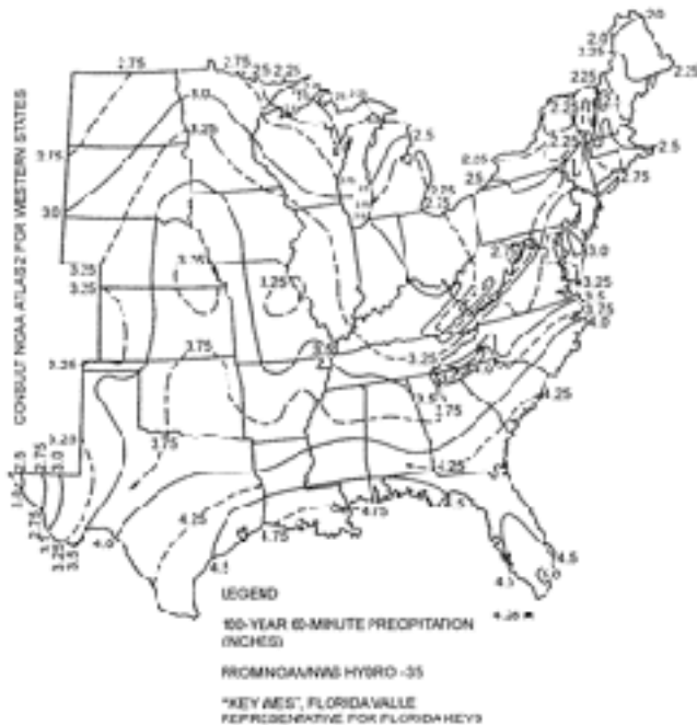
Figure 1111.E—Rainfall Rate for Primary Roof Drains (in./hr.)
